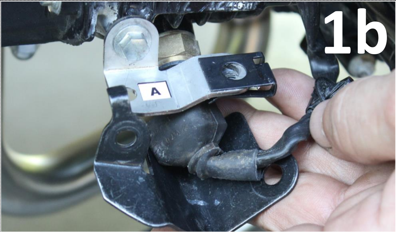
1b ) Removal of thermostat guard.
