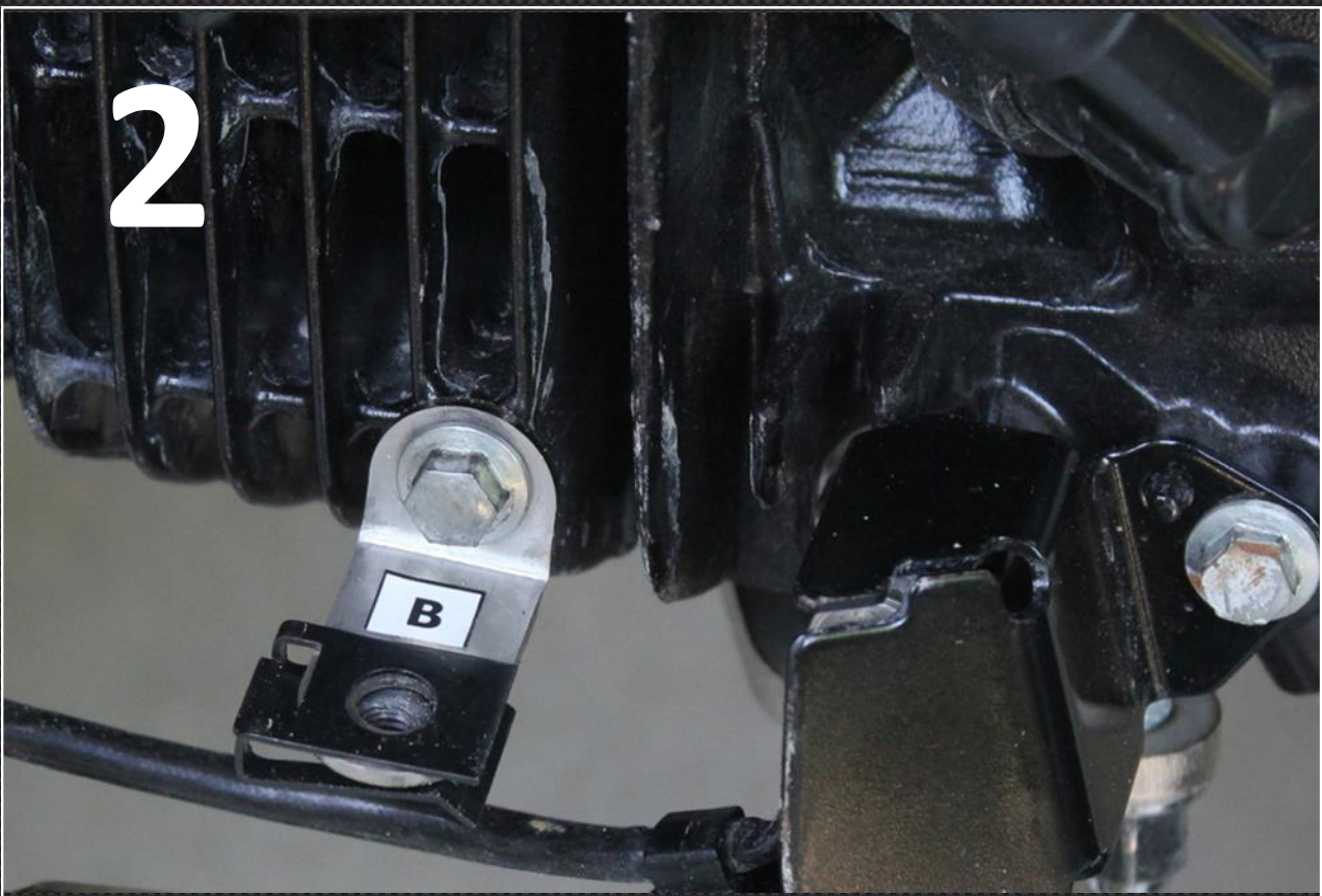
1b ) Removal of thermostat guard.
