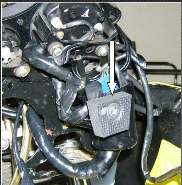
On the NC35, it is secured to the RC211V Meter stay by way of a rubber front stay and nylon bush that slips inside the main tube of the meter stay. Thread this into position on the front of the fairing before attempting to fit the front fairing to the bike.
