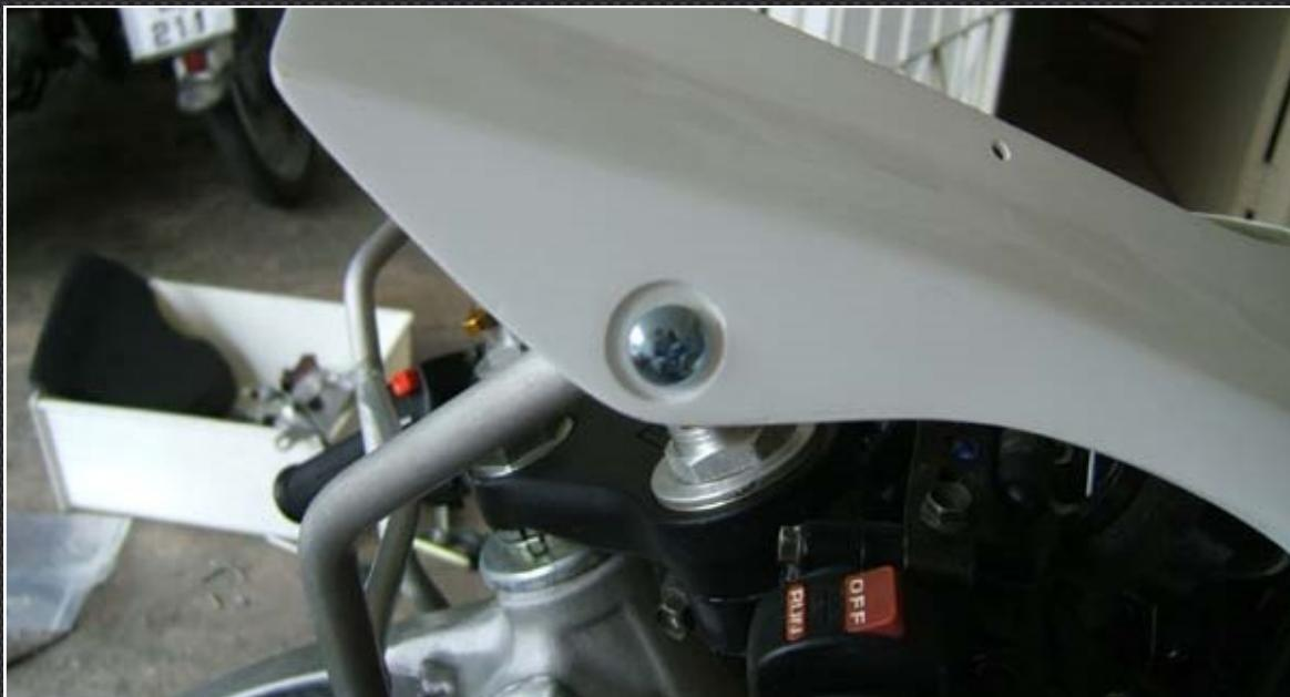
Next fit the side cowlings in position. There are four securing bolts to the front fairing for each side. Two on the outside and one each on the console and inside near the front air duct. Secure these in place.
