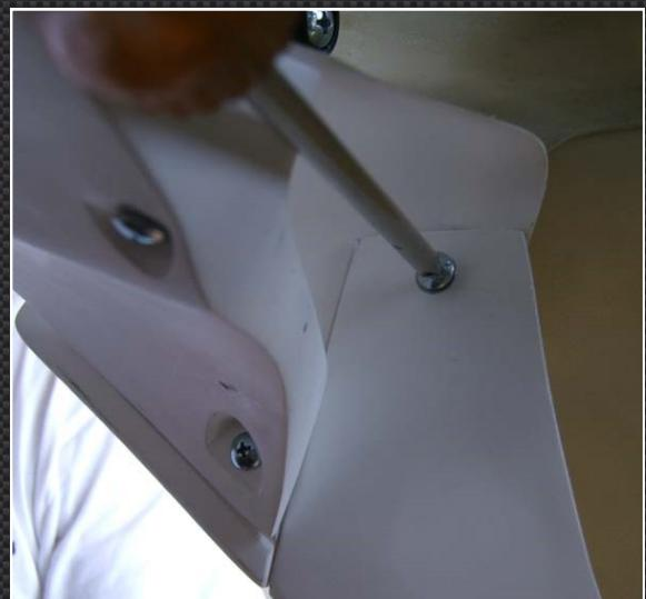
Check the alignment of the side mounting holes of the cowling with the side stays on the bike. On the NC30, don't be afraid to tweak the stay into position. On the NC35, rotate the stays into position as necessary. Secure fasteners once the stays are in position.
